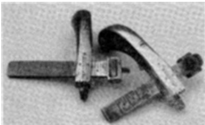
Figure 2. Two draw gauges by Henry Sauerbier; one displaying the early HENRY SOUERBIER imprint on left.
