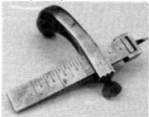
Figure 4. A draw gauge manufactured by BROWN & HAVELL.
