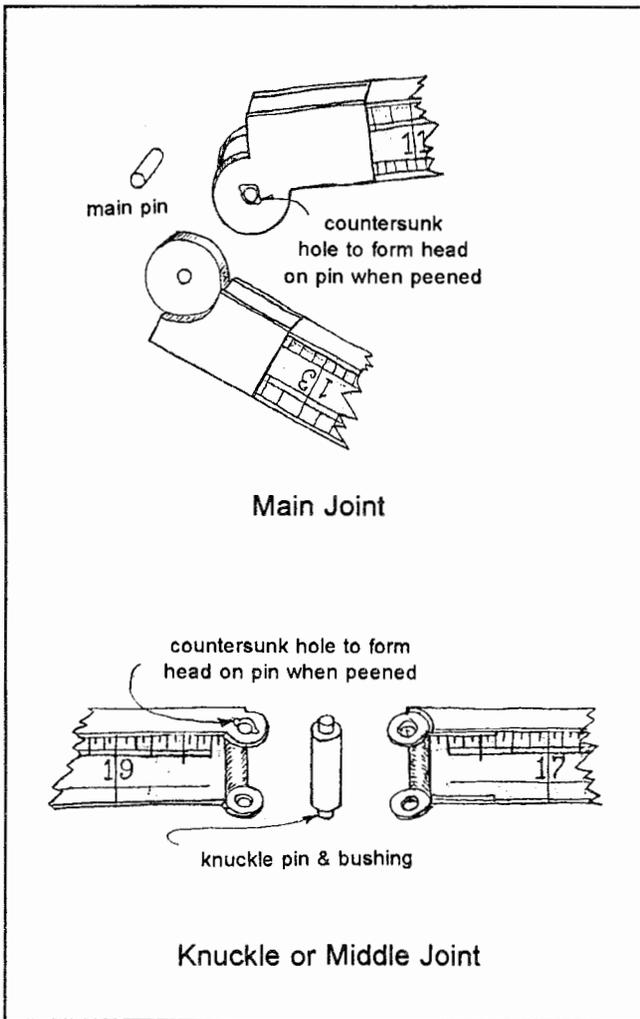
When the rule is assembled, the pins are peened into the countersunk portion of the holes. This enlarges the ends of the pin (forming heads) which prevents the pin from falling out. However, most manufacturers improved upon this simple design by forming a shape to the countersink that would prevent the rotation of the pin after peening. It is that shape that gives us a clue as to who made the rule.
