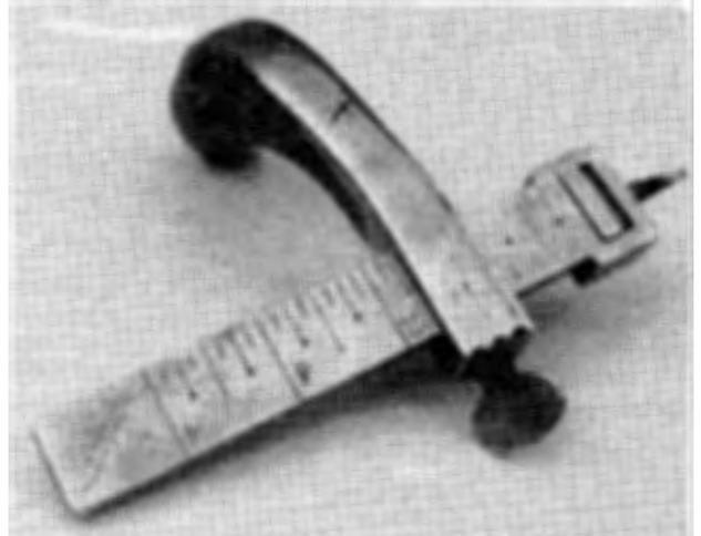
Figure 4. A draw gauge manufactured by BROWN & HAVELL.
