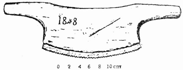
Figure 1: Croze Saws (from Woodworking in Estonia).
